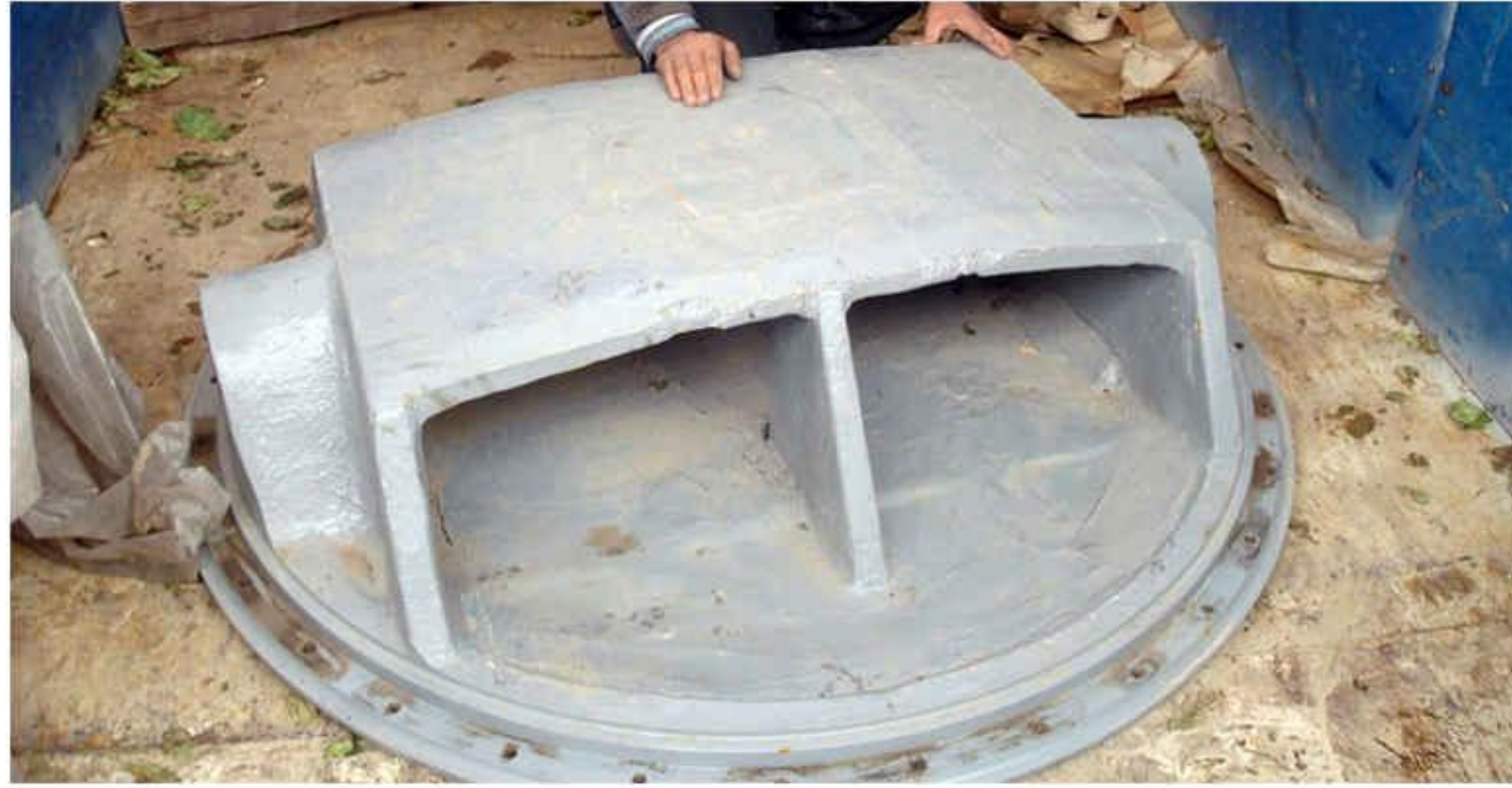
Butterfly Valve Disc 60 inch
